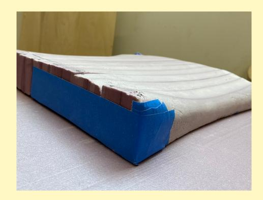
Bend study- without access to veneer, a different approach had to be made. I researched wood bending and fell upon kerf spacing to cut ply wood down to the last veneer face to allow for bends. I still wanted to make the chair out of one piece of wood as if it was molded.
