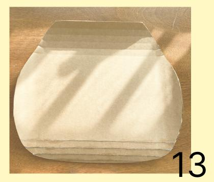
Making the mold- I spent some time shaving away at foam to form nice curvature to mold the veneer. I cut the foam into strips to form shave and then put back together.
